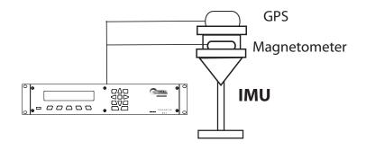
Figure 1–2. VanLink IMU Configuration
